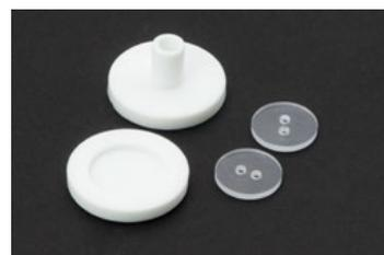
Set of two end caps of silicone for XLOOP LED tubes Ø18 or Ø25 mm, one with longitudinal access for the power supply cable, the other just a terminal element. Both the end caps are the same diameter as the LED tube and, installed on it, allow the access of the tube in different fixing and connecting accessories from the system. Sealing during installation is done with the help of liquid silicone.
