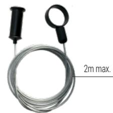
Suspension element for LED tubes with of Ø18 or Ø25 mm XLOOP, with a maximum length of 2 m. Twisted steel wire cable with die-cast aluminum fixings for ceiling and LED tube.
