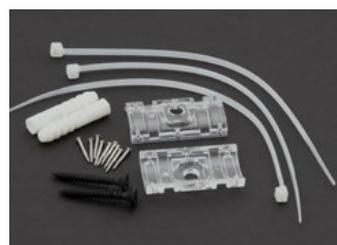
Wall or ceiling fixing system for XLOOP LED tubes Ø18 or Ø25 mm, composed of transparent polycarbonate clamp, plastic collars for temporary fixing and nails for permanent fixing.
